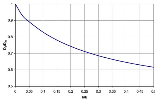
Figure 1. Optimum *Efficiency of biplane* versus  $h/b$ .
