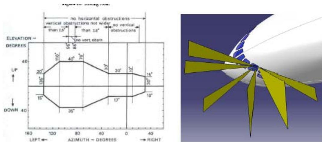
Figure 12: Vision Requirements and cockpit window solution
