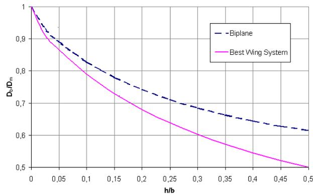
Figure 2: Induced drag of the optimum biplane/optimum monoplane rate vs h/b.
