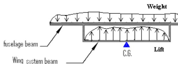
Figure 7: Structural sketch of lifting system and fuselage in a PrandtlPlane configuration.
