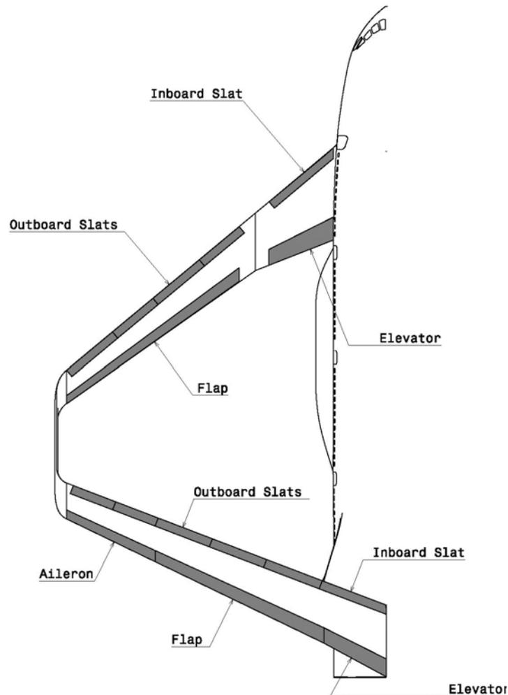
Figure 28: High lift devices and pitch control
