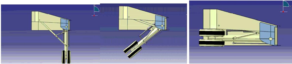
Figure 26: Kinematics of the main undercarriage
