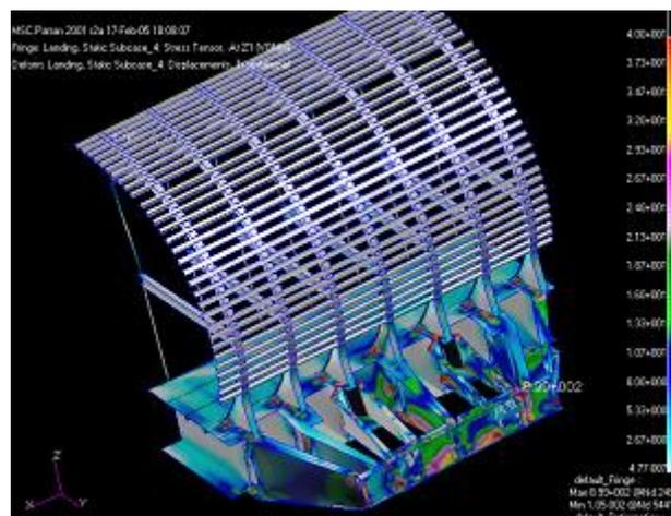
Figure 25: Finite Element model
