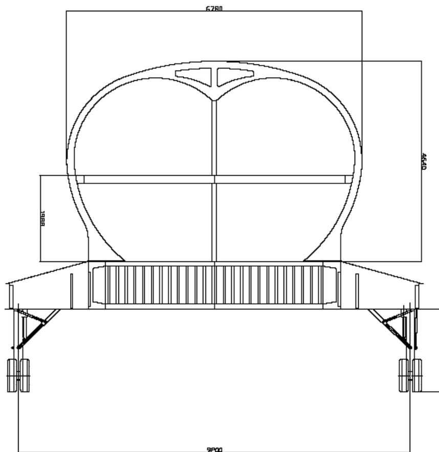
Figure 27: A sketch of the main undercarriage in the extended position.
