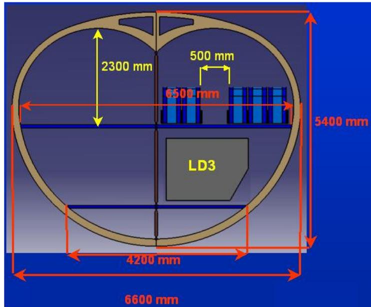
Figure 22: Sketch of the structural solution of the fuselage.
