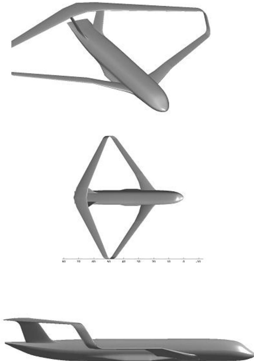
Figure 6: Sketch of a configuration with high aerodynamical efficiency and stability of flight ([8]).
