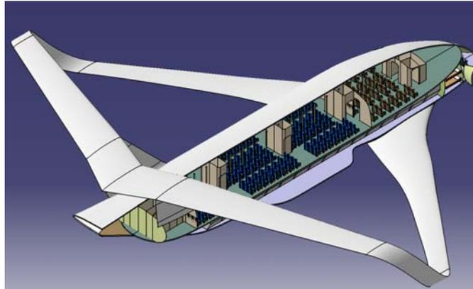
Figure 13: View of 258 passenger accommodation in two classes.
