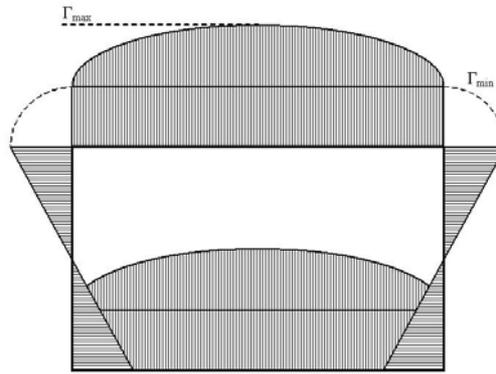
Figure 4. Lift distribution on the Best Wing System.
