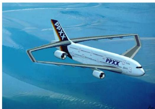
Figure 5: Preliminary application of the Prandtl's concept to transport aircraft ([6], [7]).
