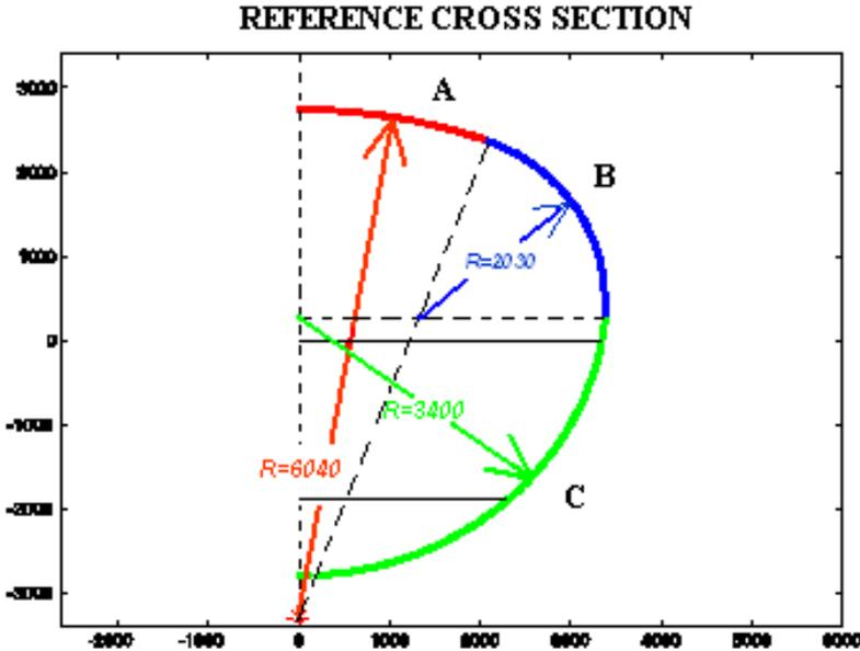
Figure 21: Outer perimeter of a typical fuselage section.
