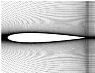
Figure 5. C-topology grid for the plunging NACA0012 airfoil
