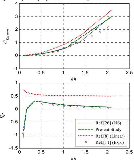
Figure 7. Variation of  $C_{Tmean}$  and  $\eta_p$  with  $kh$  at constant  $h = 0.175$
