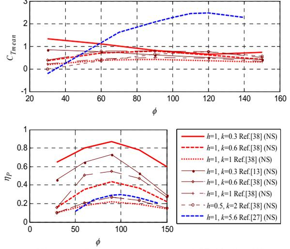
Figure 4. Variation of  $C_{Tmean}$  and  $\eta_P$  with  $\phi$  of 2D NACA0012 airfoil undergoing combined plunging and pitching motion.
