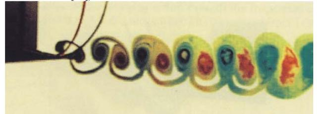
Figure 2. Thrust producing wake for a NACA0012 airfoil undergoing pure plunging motion,  $h = 0.025$ ,  $kh = 0.393$  (From Lai and Platzer [21])
