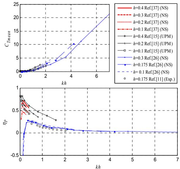
Figure 3. Variation of  $C_{Tmean}$  and  $\eta_P$  with  $kh$  of a 2D NACA0012 airfoil undergoing pure plunging motion
