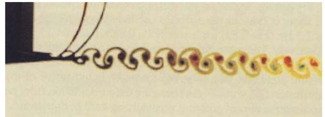
Figure 1. Drag producing wake for a stationary NACA0012 airfoil (From Lai and Platzer [21])
