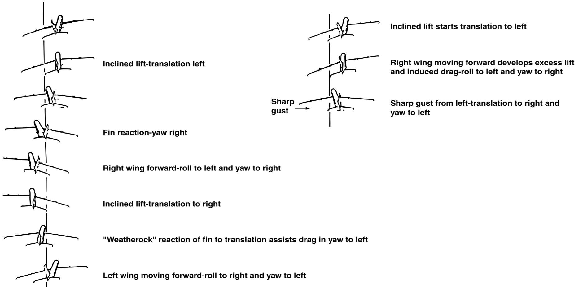
**First cycle of a typical dutch roll development as viewed from AFT and above the airplane**
