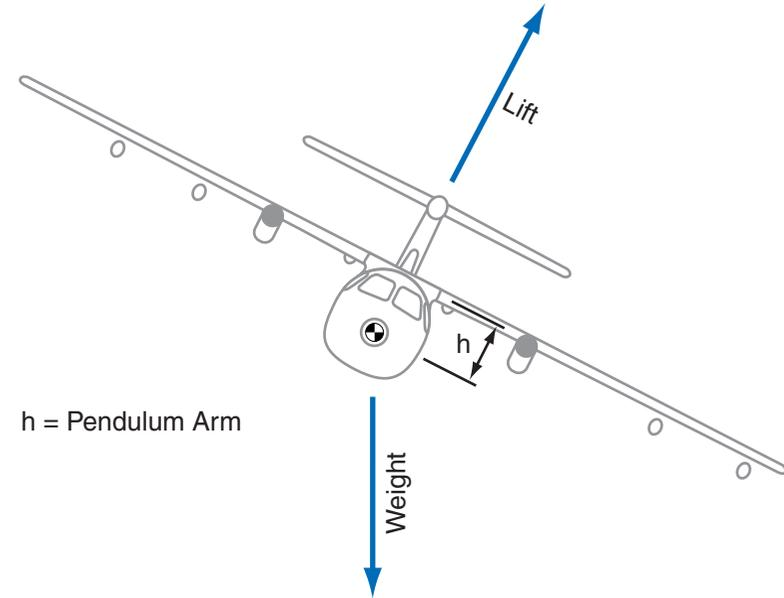
If an aircraft is very stable directionally and not very stable laterally, e.g. if it has large fin and rudder and little or no dihedral angle, or other “dihedral effect”, it will have a marked tendency to turn into a sideslip, and to bank at steeper and steeper angles, that it may get into an uncontrollable spiral this is sometimes called spiral instability, but note that it is caused by too much stability (directional).
